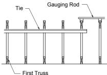
Locate and space each truss using Gauging Rod
